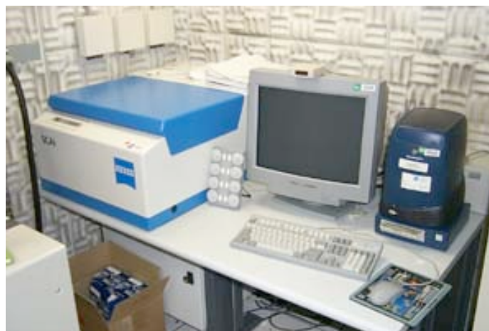
Fig. III.86. The Zeiss Photoscan densitometer is generally used to scan images at a pixel step size of 7 \mu\text{m} . (From Scripps Research Institute CIMBio web site)
