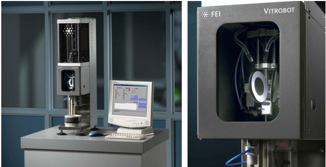
Fig. II.71. Vitrobot plunge freezing device sold by FEI Company. The device allows samples to be vitrified under controlled temperature and humidity conditions. Such control provides a means to achieve greater reproducibility in freezing experiments. (From FEI Brochure)
