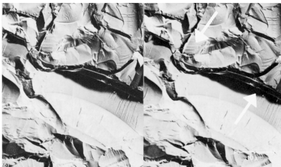
Fig. I.172. Stereoscopic pair of shadow cast, two-stage replica of a diamond-ground glass surface. (From Watt, 1985, p.138)
