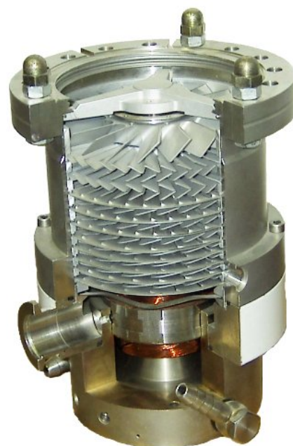
Fig. I.95. Interior view of a turbomolecular pump. (From http://en.wikipedia.org/wiki/Turbomolecular_pump )
