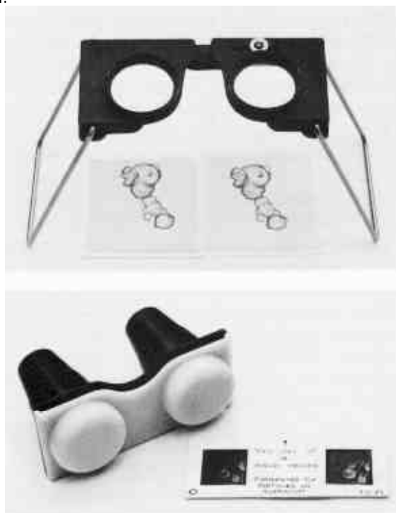
Fig. I.173. Simple viewers for stereoscopic pairs. 'Spectacles on stilts' enable a pair of prints up to 6.3 cm wide to be seen, enlarged, in 3D. The separation between the two halves of the viewer can be varied to accommodate differences in interocular separation between observers. The molded plastic transparency viewer accepts pairs of transparencies in 4.25 x 10.1 cm cardboard or metal frames. (From Watt, p.136)
