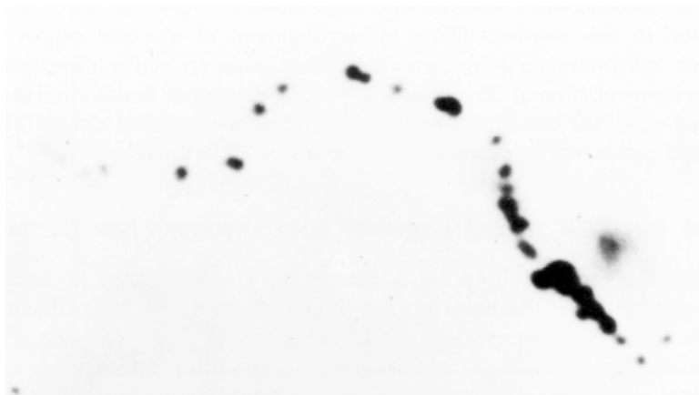
Fig. I.150. Photomicrograph of the track of an electron having an initial energy of 75keV recorded in a nuclear track type emulsion layer. The dense aggregation of grain occurs towards the end of the track. Magnification ~4,500X. (From Farnell and Flint, p.23)
